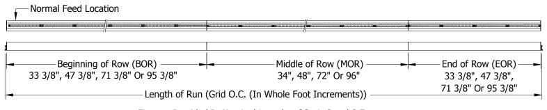
Fixtures Provided In Nominal Lengths of 3, 4, 6 and 8 Feet. (Depending upon Job-Site Capacity, Fixtures Can Be Provided In Longer, One Piece Lengths (Consult Factory))
