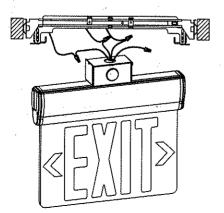
4. Snap unit on the bar hanger, spring clip will hold the unit.
