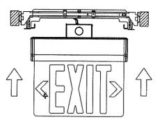
Fix LED indicator holder, LED indicator and test switch on the trim plate, connect test switch connector.
