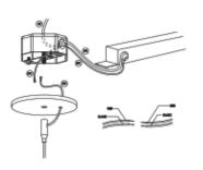
Fasten the MIDDLE OF RUN (MOR) fixture to the EOR fixture by engaging it into the Joiner Bracket. Lightly engage (1) Set Screw if needed. Secure the Power End of the fixture to the ceiling (Ref Step 2). Tighten the Set Screws in the joiner.
