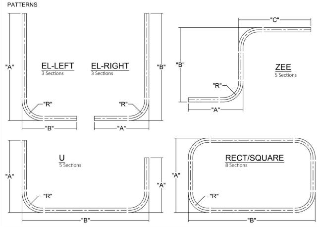
Curved Patterns may consist of straight profiles and curved profiles or just curved profiles. All match in profile.
